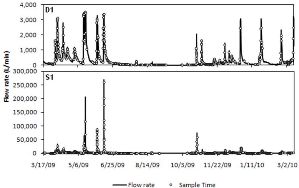
Figure 2. Hydrograph and corresponding sample times at D1 (top) and S1 (bottom). Each dot represents a 1-L grab sample collected by an ISCO automated sampler.
