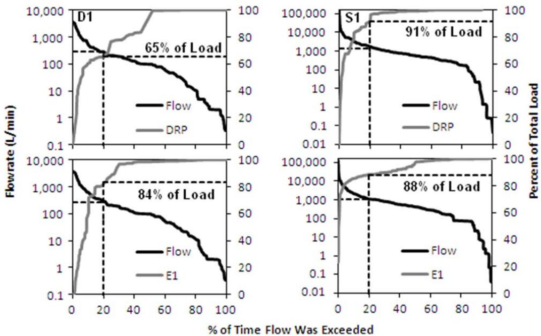
Figure 4. Flow duration curves and cumulative load plots at D1 (right) and S1 (left).
