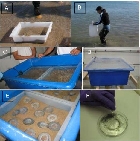
Figure 1 Set up of diffusion chambers and simulated natural environment. (A) Field collection of sediment. (B) Field collection of water using 25L carboys. (C and D) Simulated natural environment set up in laboratory using collected Lake Michigan sediment and water. (E) Diffusion chambers incubated on the surface of the sediment. (F) Diffusion chamber being opened for observation after incubation in the simulated natural environment. Results:
