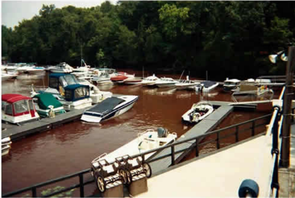
Figure 1. View of the embayment during the 2002 dye study. The water is pink because of Rhodamine WT dye that was injected in the main channel and trapped in the embayment.
