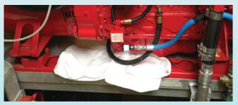
Oil absorbent booms, sheets (bottom), and pads can be kept on your boat to catch leaks under the engine or to contain and remove oil at the surface of the water (back). Bilge socks (top) trap any oily overflow on board, making safe disposal easy. (MASGC/Tara Skelton)
