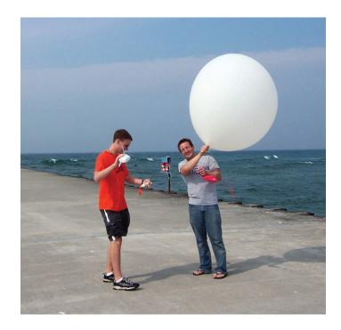
The device they used is called a rawinsonde, which is attached to a weather balloon with a parachute. Because the system is connected to a balloon, researchers were also able to record the wind direction and speed.
