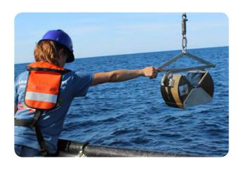
The PONAR grab is used to capture organisms and sediment from the lake bottom.
